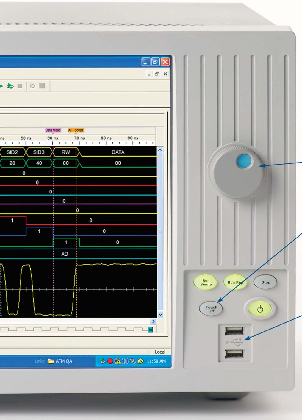
**General-purpose knob** lets you quickly adjust your viewing and measurement parameters. Select a modifiable variable, then turn the knob to quickly step through values for the variable.
